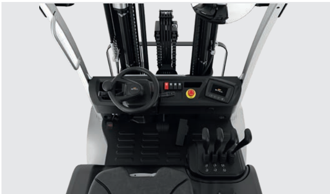
Flexible and comfortable: the operator's seat and steering column are infinitely adjustable, so that the cab can be quickly and easily adjusted for operators of different heights
