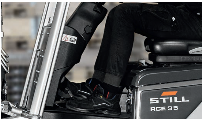
The RCE has a spacious footwell, which ensures an ergonomic seating position and allows for easy access
