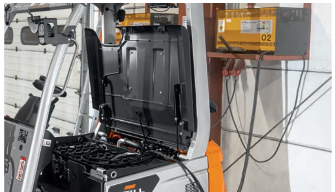
Thanks to the compact STILL charging station, decentralised charging of the battery is also possible
