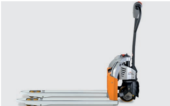
Compact design of a hand pallet truck for working in confined spaces
