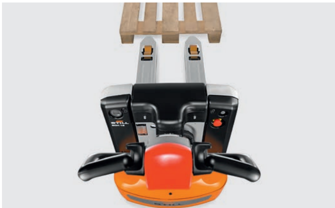
The low height of the pallet truck makes the fork tips easy to see
